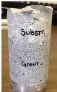
A. Mode 1: Substrate failure.
