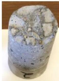
B. Mode 2: Bond failure at the interface.
