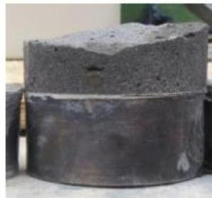
C. Mode 3: Failure in the bonded material.
