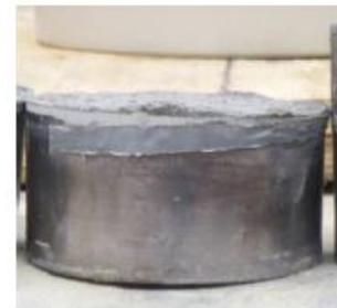
D. Mode 4: Failure in the disc adhesive.
