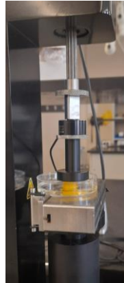
Figure 6. Arrangement of the samples in the compression test machine.
