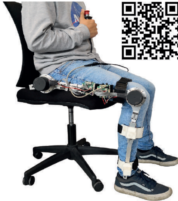
Figure 5.4: Stationary therapy of the AGoRA exoskeleton. This approach was undertaken to prove the effectiveness of the transparent mode in terms of the actuator position and velocity. Scan the QR code to watch a demonstration video of this stationary approach. In case you are unable to scan such code, click here: https://www.youtube.com/watch?v=eseWTEUN3e4 .
