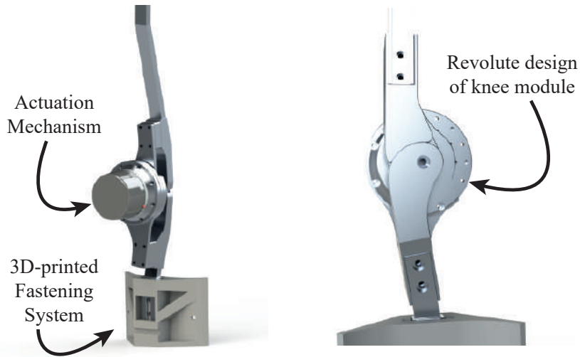
Figure 3.3: Knee module of the AGoRA exoskeleton. A 3D-printed fastening system ensures proper torque transmission of a motor-gearbox construction which serves as actuation mechanism on the exoskeleton knee module.
