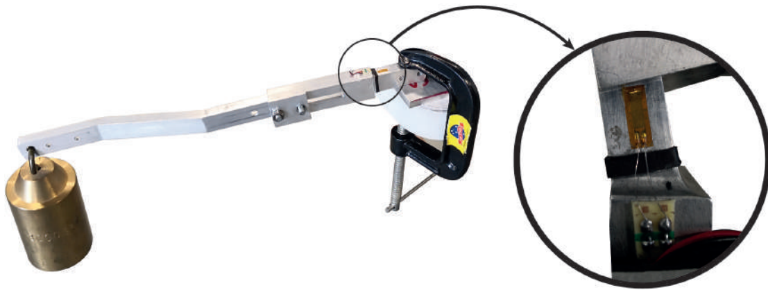
Figure 3.7: Strain gauge calibration setup. A set of calibrated weights was used to model an estimation of the interaction torque.
