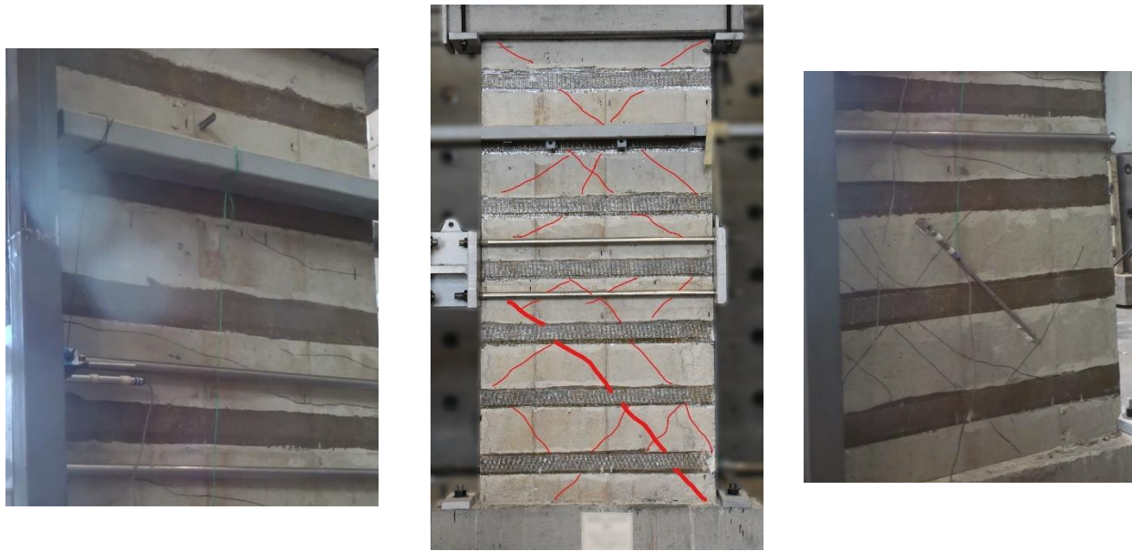
Figure 4.4 – Failure mode L-G1-2 Specimen.
