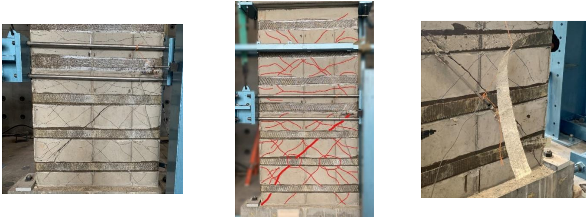
Figure 4.11 – Failure mode H-G1-2-90 Specimen.
