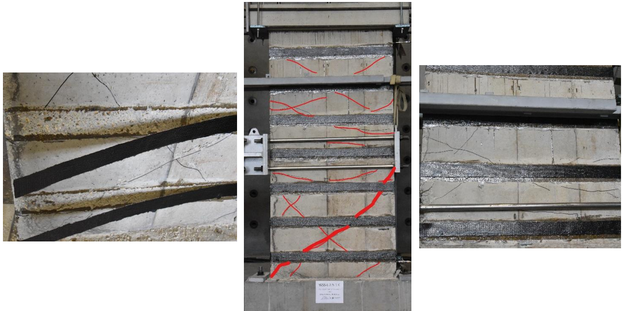
Figure 4.5 – Failure mode L-C1-1 Specimen.
