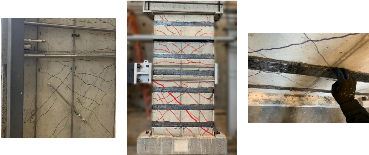
Figure 4.9 – Failure mode H-C21-1 Specimen.
