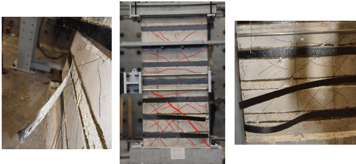
Figure 4.6 – Failure mode L-C1-2 Specimen.
