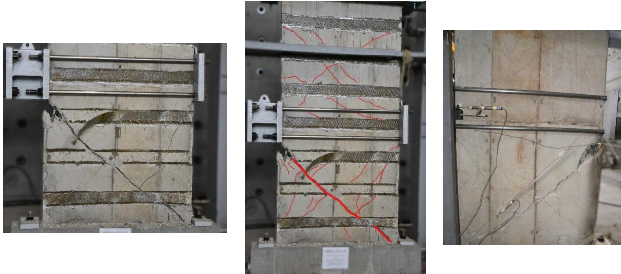
Figure 4.3 – Failure mode L-G1-1 Specimen.
