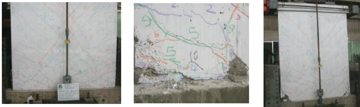
Figure 2.3 – Failure mode RC walls
