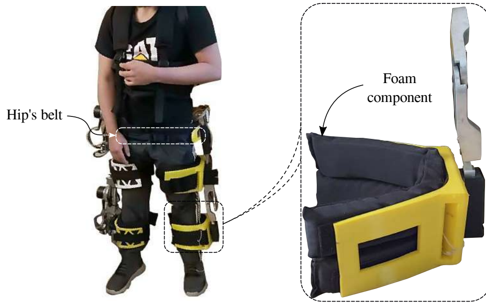
Figure 5.1: AGoRA physical interfaces' third version. The latest physical interfaces' version including the hip belt and additional foams.
