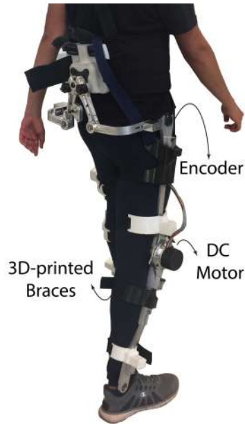
Figure 3.5: AGoRA-LLE's physical interfaces first version. An overlapped version of physical interfaces made of 3D printed Nylon, fabric, and fastener.
