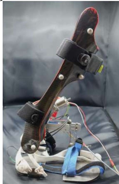
Figure 2.11: A customized physical interface for an ankle-foot orthosis. Extracted from [69]. A. The 3D scanner of the user's limb and CAD model for the physical interface. B. The customized physical interface to a powered ankle-foot exoskeleton.
