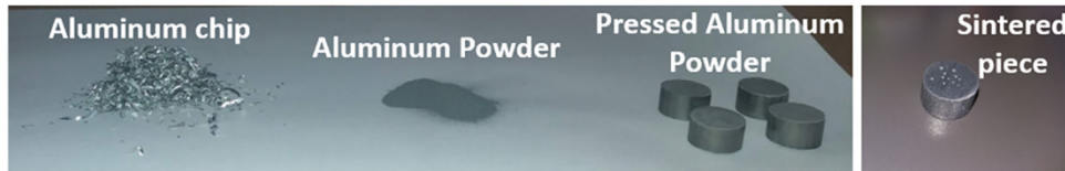
Fig. 1 – Transition from chips to sintered pieces (sintered pieces are showing indentations on its surface).
