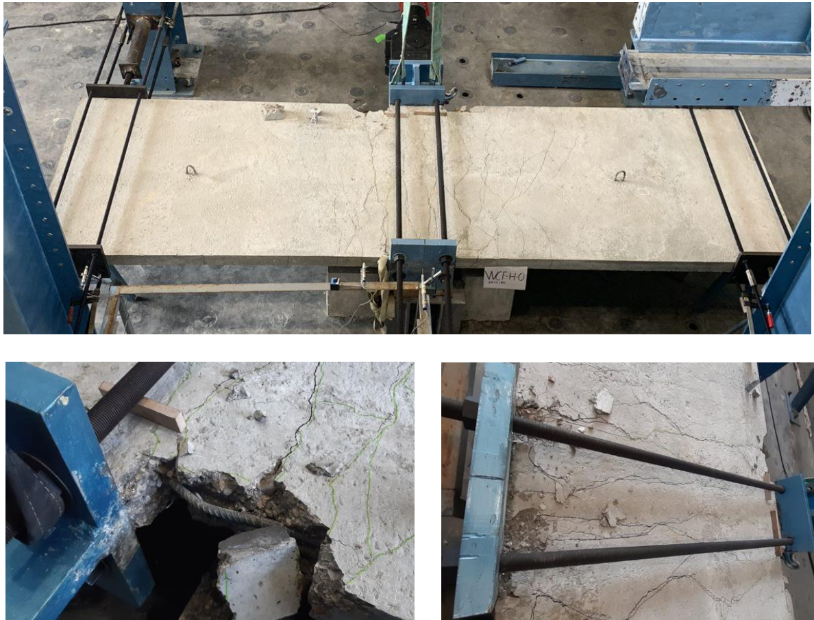
Figure 5-6 Failure mode H-0 Specimen Own source
