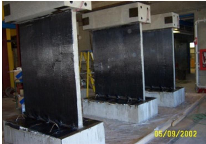
Figure 2-1- Tests for specimens' strengthening with FRP bands on both sides of the wall Source: Cruz-Noguez et al., 2015
