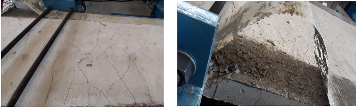
Figure 5-3 Failure mode L-GHS-1 Specimen.
