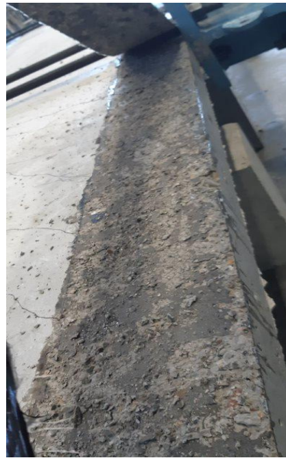
Figure 5-5 Failure mode L-CHS-2 Specimen.
