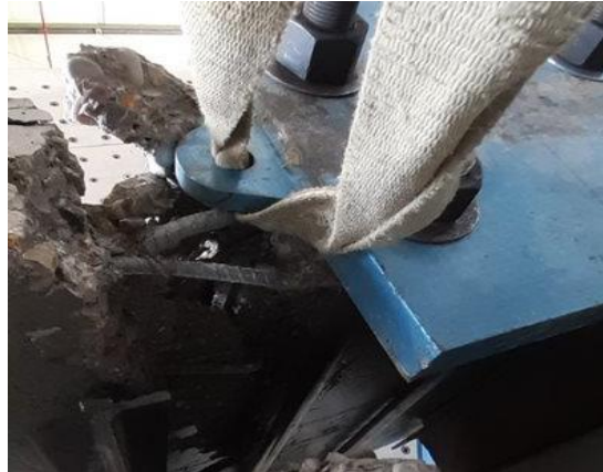
Figure 5-2 Failure mode L-0 Specimen. Own source
