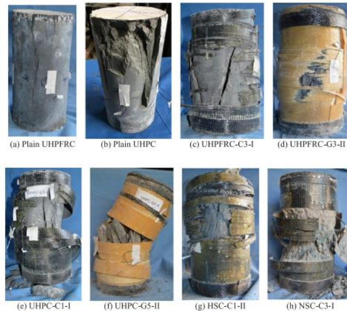
Figure 58. Specimens' mode of failure. By: Wang.
