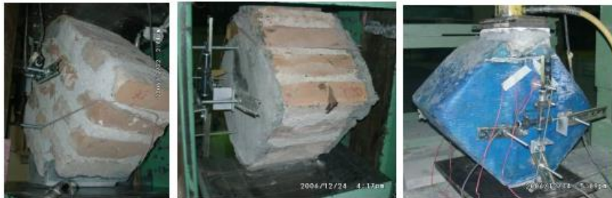
Figure 23. Reference (type A) plastered (type B) & retrofitted (type C) specimens. By: Ilki.
