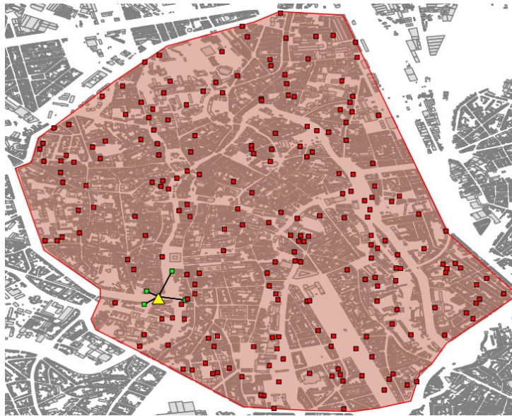
Figure 5.4: Example of an EIRP PwrC Opt network with only one UABS (yellow triangle). Only a very few users (green) are connected. All other users (red) remain uncovered.
