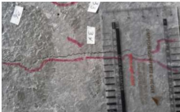
Figura 7. Fisura de espesor mayor a 0.4mm. Fisura # 28 M 2-18-C-0 (04 abr/14)
