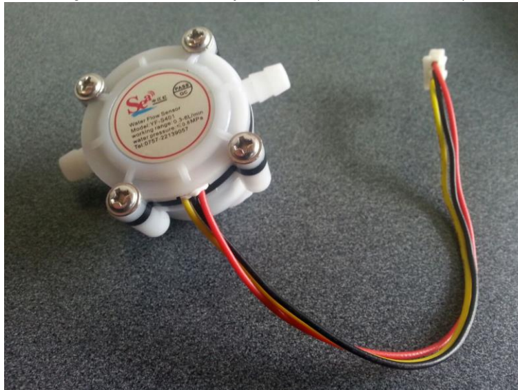
Figura 66. Sensor de Flujo YF-S401 (4.5 ml/s – 100 ml/s)
