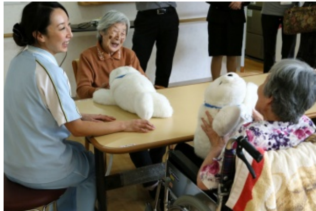
Figure 3.3: Paro robot in an Elderly Care Center. This robot is mostly used to treat the dementia and the mental healthcare of the elderly [65].
