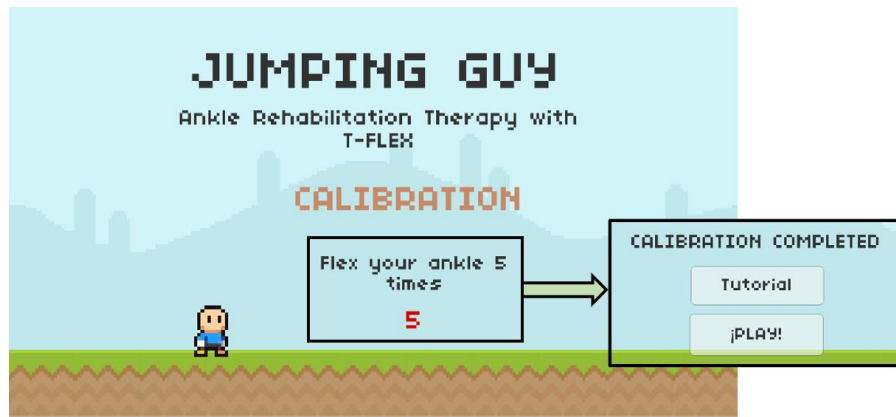
Figure 28. Calibration Interface. The box on the right corresponded to the messages and buttons activated after completing the task.
