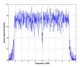
Fig. 2. Spectral power density of an OFDM 8K with FFT processing, Eb/No= 10 (dB) and guard intervals Δ=Tu/4 AWGN (10dB). Source: Matlab®, Authors.
