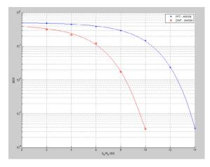
Fig. 4. BER values with relations Eb/No from 1-14dB to channels AWGN. Source: Matlab®, Authors.
