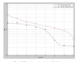
Fig. 7. BER values with relations Eb/No from 1-14dB for RICIAN channels Source: Matlab®, Authors.
