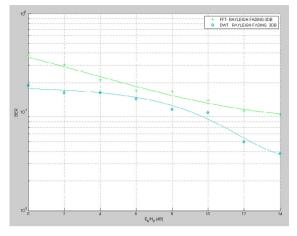
Fig. 6. BER values with relations Eb/No from 1-14dB for RAYLEIGH channels. Source: Matlab®, Authors.
