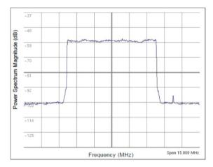
Fig. 3. Spectral power density of an OFDM 8K with DWT processing, and Eb/No= 10 (dB). Source: Matlab®, Authors.
