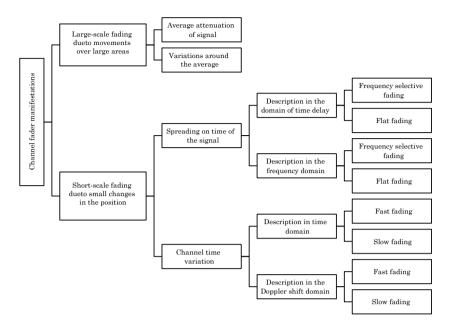
Fig. 1. Fading types in a wireless channel. Source: Authors.
