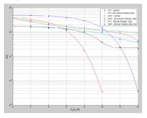
Fig. 8. BER values with relations Eb/No from 1-14dB for AWGN, RAYLEIGH, and RICIAN channels. Source: Matlab®, Authors.
