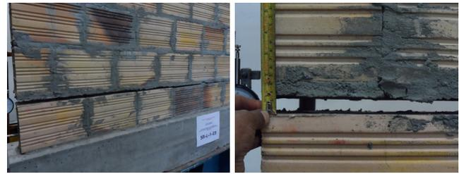
**Figure 7.** Failure mode of the URM walls.
