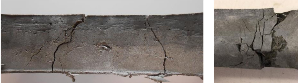
Figure 16. Multi-cracking pattern in the experimental validation specimen gage.
