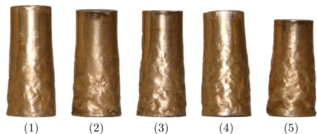
Fig. 9 Taylor specimens after impact. Impact velocity: (1) 101.56 m/s, (2) 112.87 m/s, (3) 123.70 m/s (4) 131.47 m/s (5) 177.80 m/s
